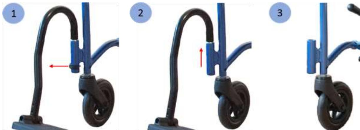
The plastic footrest tray can be adjusted in height to allow the user maximum comfort. The small bolt can be removed from the base of the plastic footrest tray and re-inserted into one of the three possible elevation holes on the footrest tube by using the Allen wrench provided with the wheelchair.
